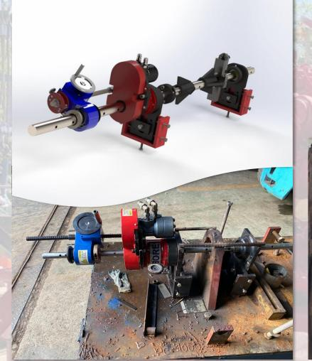
A more compact and affordable version of line boring machine, with the mounting flexibility needed for work in restrictive spaces. A variety of motor and bar options add power to this outstanding value. Used for stern tubes, rudder bores, track pad, bucket excavator, hinge pins, gearboxes, turbines, and many more applications
